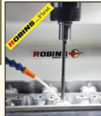
Guide honing up to 0.006" (single cycle) eliminates reaming
