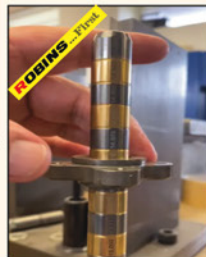
Custom Master gages for precise bore size and taper measurement.. accurate within 0.0001"
