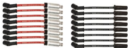
Part Nos. 73740 - 73747 Ultra 40 Wire Set, 8.5mm, 1S Options: Red/Black, With or W/O Heat Shields, 9.75" or 11" Long
