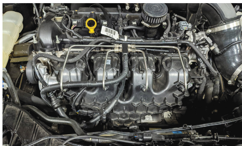
Pictured here is a Ford 2.3-liter EcoBoost engine outfitted with direct-port methanol injection. The addition of fuel from an auxiliary source helps reduce demand on the factory fuel system.
