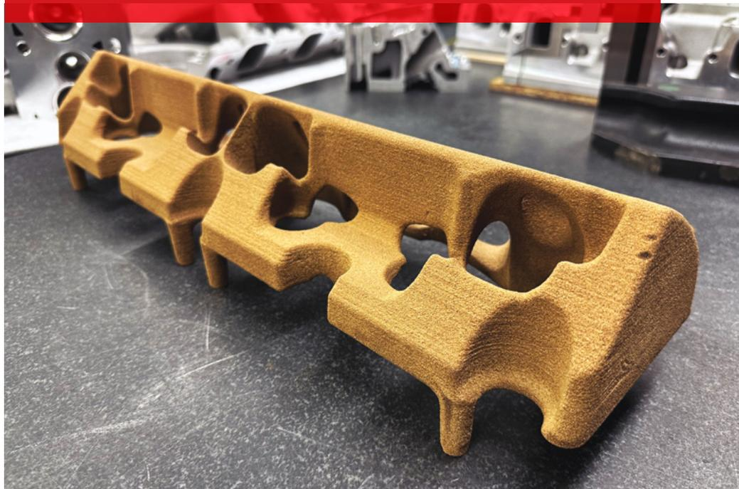
tolerances. While current 3D printers can achieve mathematically complex surfaces, the resolution doesn't always meet the engineers' requirements.
