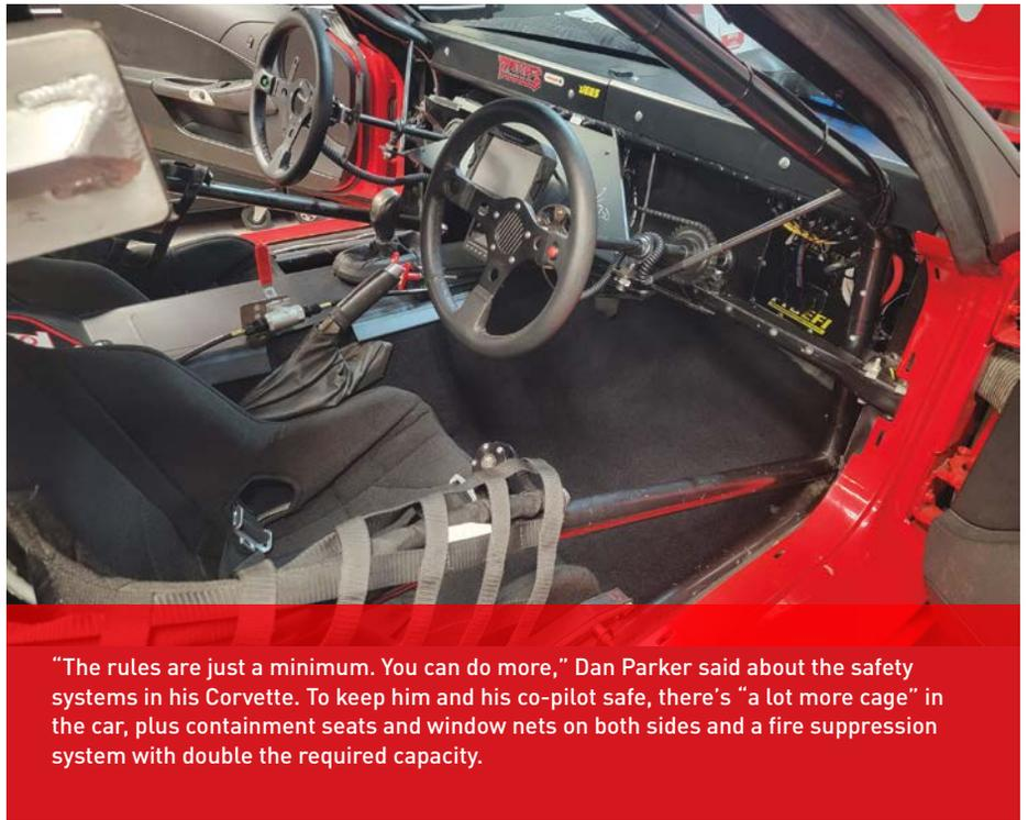
“The rules are just a minimum. You can do more,” Dan Parker said about the safety systems in his Corvette. To keep him and his co-pilot safe, there’s “a lot more cage” in the car, plus containment seats and window nets on both sides and a fire suppression system with double the required capacity.
