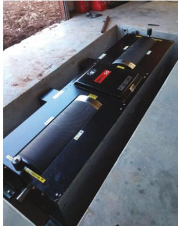
Regular cleaning also provides opportunities to lubricate the bearings and eddy current brakes. "Make sure to use the lubricant that's recommended by the dyno manufacturer and follow the recommended lubrication schedule," Caldwell said. Owners should keep in mind that those schedules can vary widely depending on a dynamometer's design.
