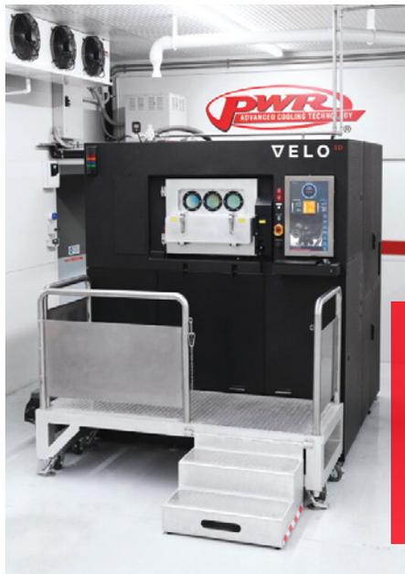
Here is the Velo3D Sapphire printer used by PWR. This laser powder bed fusion printer works by selectively welding 50-micron layers of metal powder to produce a final part that is then heat-treated and machined.
