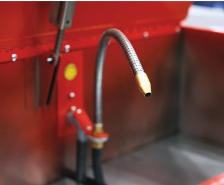
When using parts cleaning equipment with nozzles, like this Safety-Kleen cabinet, it's important to have a good filtration system, one of our sources said. That will prevent debris clogging the nozzles, which will keep the equipment running efficiently.
