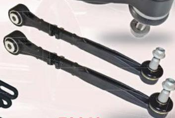
SPC's 6-arm set, part #72600 includes a pair each of the #72610, #72630 and #72640 arms. All performance arms feature OE sized, high durometer bonded rubber bushings with rebuildable ball joints and Trailing Links feature SPC xAxis™ sealed flex joints. All arms feature strong 6061-T6 forged aluminum castings with anodized finish for performance you can feel.
