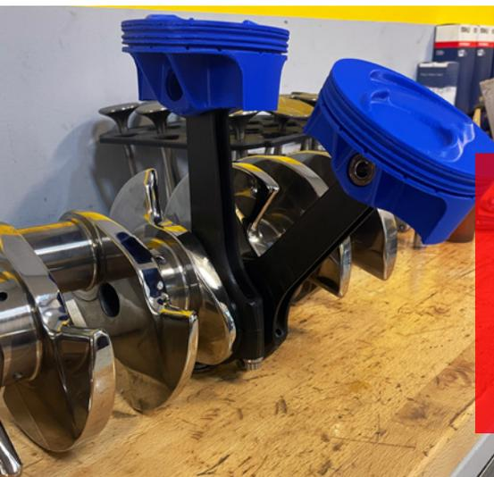
Ben Strader of EFI University uses 3D-printed parts for mock-up purposes to check clearances and fitment before ordering the actual components. "We aren't big enough to justify the expense of owning the machines," he explained, but there are plenty of parts manufacturers that offer this service to his shop.
