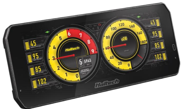
aftermarket ECU brands. It offers plenty of scope for sensors and other inputs in standalone or for use as an I/O expander in a Haltech environment. The uC-10 has the same mounting points as the iC-7, so an upgrade is quite easy, and it fits a variety of dash profiles.
