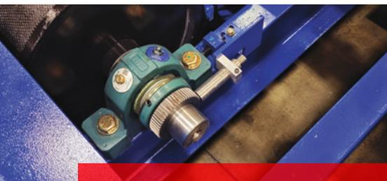
Shown here is a Mustang Dynamometer speed sensor and toothed gear. Michael Caldwell said the gear should be "clean and free of any dust or tire debris." Also visible in the photo are pillow block bearings, which should be greased per the instructions that came with the dynamometer.
