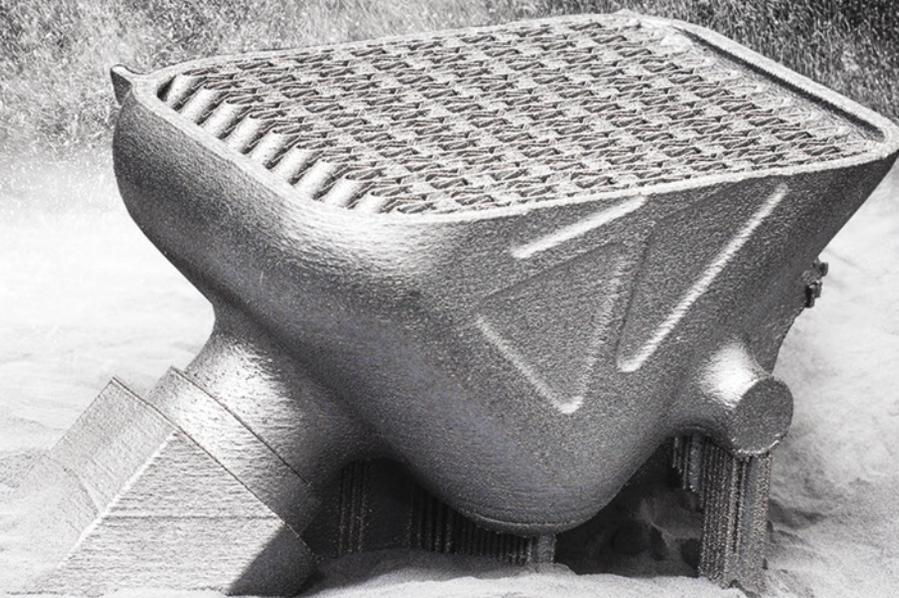
The mid-July summer heat of 2020 was unbearable for IndyCar drivers at the Road America double-header. The new Aeroscreen protection reduced cockpit air circulation, so teams, race officials, and engineers from vehicle designer Dallara collaborated on ways to introduce a fresh-air cooling duct. Time certainly wasn't a luxury as a pair of 250-mile races was scheduled for the following weekend in the sweltering Midwest.
