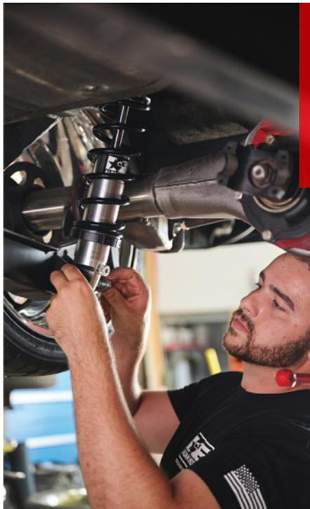
Aldan American's drag racing coilover systems are commonly used in index classes for their consistency and ability to be adjusted for track conditions to run specified ETs. Aldan has also released products for cruise-night cars that occasionally autocross.
