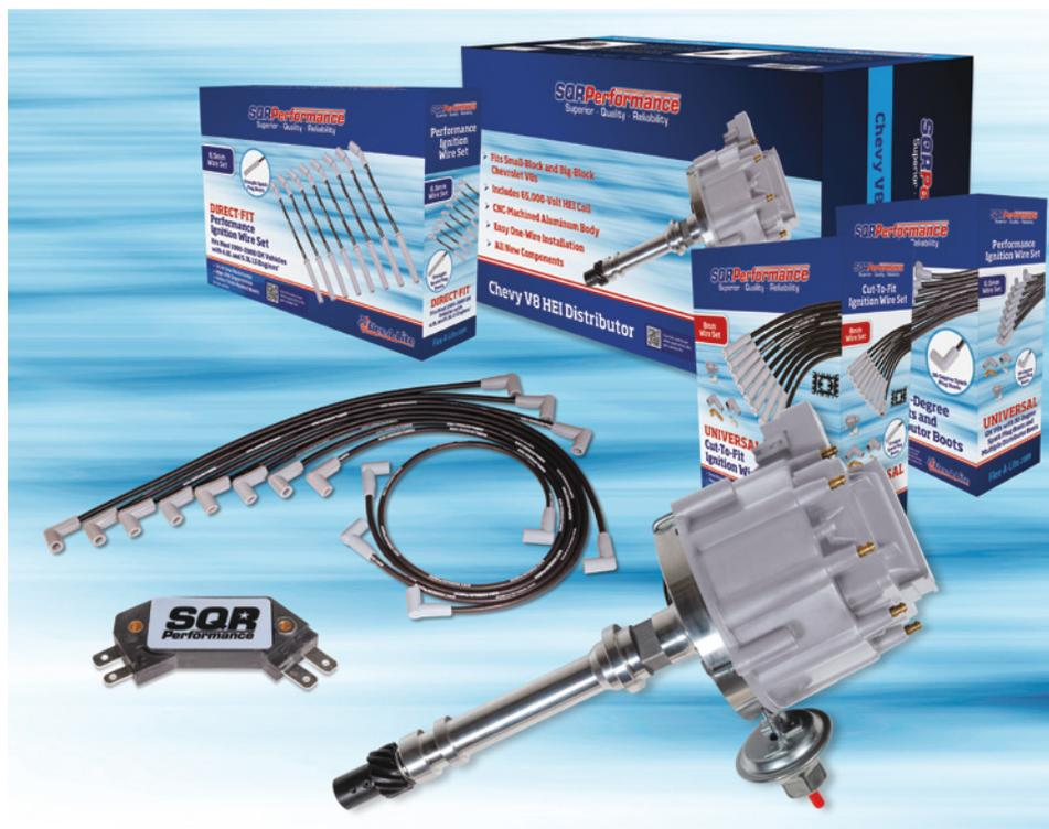
the cap, and an SQR Performance HEI ignition module. It also comes with a mild performance mechanical advance timing curve, and the vacuum advance is easily adjusted. The four-pin module provides high coil output and is constructed from solid state electronics.
