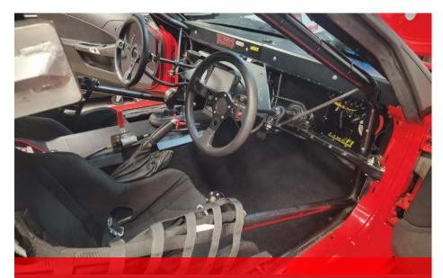
"The rules are just a minimum. You can do more," Dan Parker said about the safety systems in his Corvette. To keep him and his co-pilot safe, there's "a lot more cage" in the car, plus containment seats and window nets on both sides and a fire suppression system with double the required capacity.
