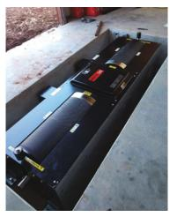
Regular cleaning also provides opportunities to lubricate the bearings and eddy current brakes. "Make sure to use the lubricant that's recommended by the dyno manufacturer and follow the recommended lubrication schedule," Caldwell said. Owners should keep in mind that those schedules can vary widely depending on a dynamometer's design.
