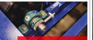
Shown here is a Mustang Dynamometer speed sensor and toothed gear. Michael Caldwell said the gear should be "clean and free of any dust or tire debris." Also visible in the photo are pillow block bearings, which should be greased per the instructions that came with the dynamometer.
