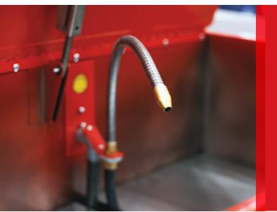
When using parts cleaning equipment with nozzles, like this Safety-Kleen cabinet, it's important to have a good filtration system, one of our sources said. That will prevent debris clogging the nozzles, which will keep the equipment running efficiently.
