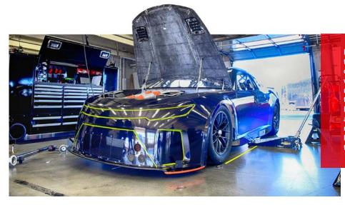
From the independent rear suspension to the rear diffuser and single lug-nut design, NASCAR's Next Gen Cup car was designed "with an eye for how relevant the car topology is to the rest of the world," said NASCAR Chief Racing Development Officer John Probst. More akin to traditional GT cars, "the idea was not only to attract new [team] owners," but also "to attract drivers from all over the world."
