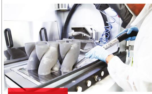
A section of exhaust for a Porsche GT2 RS car is 3D printed at Pankl. Here, the employee is vacuuming up leftover metal powder that can then be recycled.
