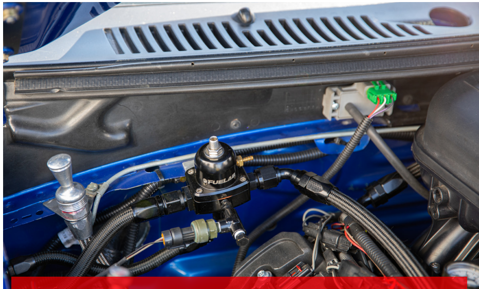
An electronic fuel pressure regulator is used to control the speed of a brushless electric fuel pump based on the demand that the system senses.
