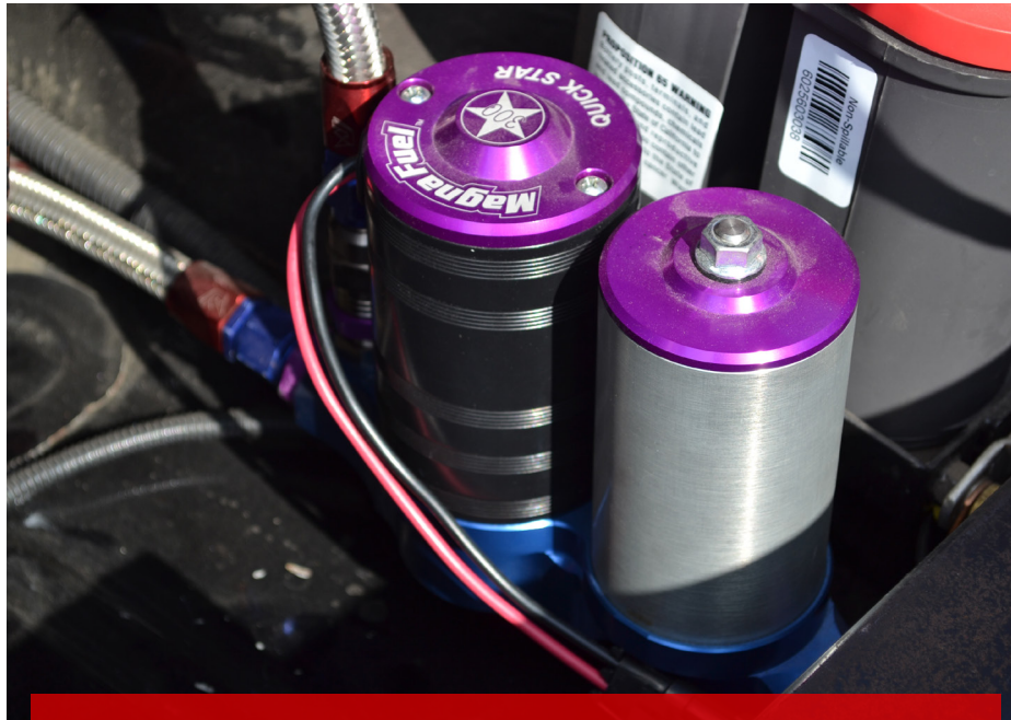
MagnaFuel external fuel pumps can be purchased with a companion fuel filter, as shown here, or without one. The QuickStar model can support more than 950 hp.
