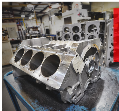
Brodix has developed a small block Chevy block with the camshaft raised to the height of a big block Chevy. This block also takes a BBC front drive.
