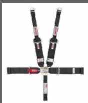
These 2-inch upper shoulder belts fit better with a head-and-neck restraint.
