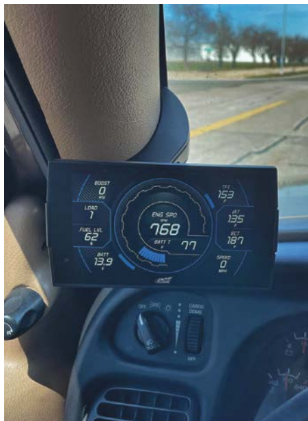
Edge Products' Insight CTS3 on-dash monitor provides drivers with real-time data that includes transmission fluid and coolant temperatures, engine oil and exhaust gas temperatures, boost pressures, and more.
