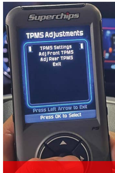
Superchips' hand-held tuners enable the driver to perform multiple functions, not all of them related to engine performance. Some models enable the driver to adjust the Tire Pressure Management System engagement threshold or bypass it entirely.
