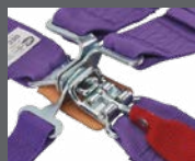
Speedway Motors' five-point harness latch collects all five belt segments.
