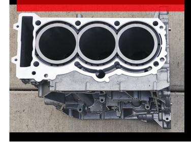
engine in Can Am vehicles. A MID conversion involves turning a dry-liner engine into a wet-liner configuration.
