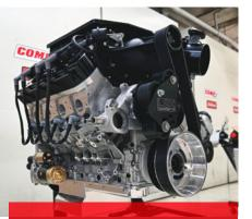
The LS engine block offered by RHS was built to withstand extreme boost by utilizing premium aluminum in its construction and six-bolt steel main caps, which are designed for increased clamping strength.
