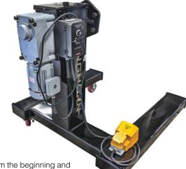
"We started from the beginning and redesigned the whole concept of how we rotate engines," said Manfred Schreyer, "much of which is side mounted to allow an engine to be bolted to the stand by only taking off one motor mount."
