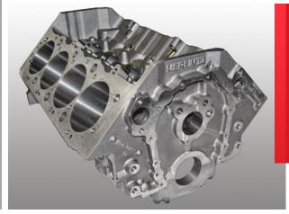
World Products offers a BBC block with a 9.5-inch deck height. "The shorter deck allows racers to keep the rotating assembly lighter and the center of gravity lower," said our company source.
