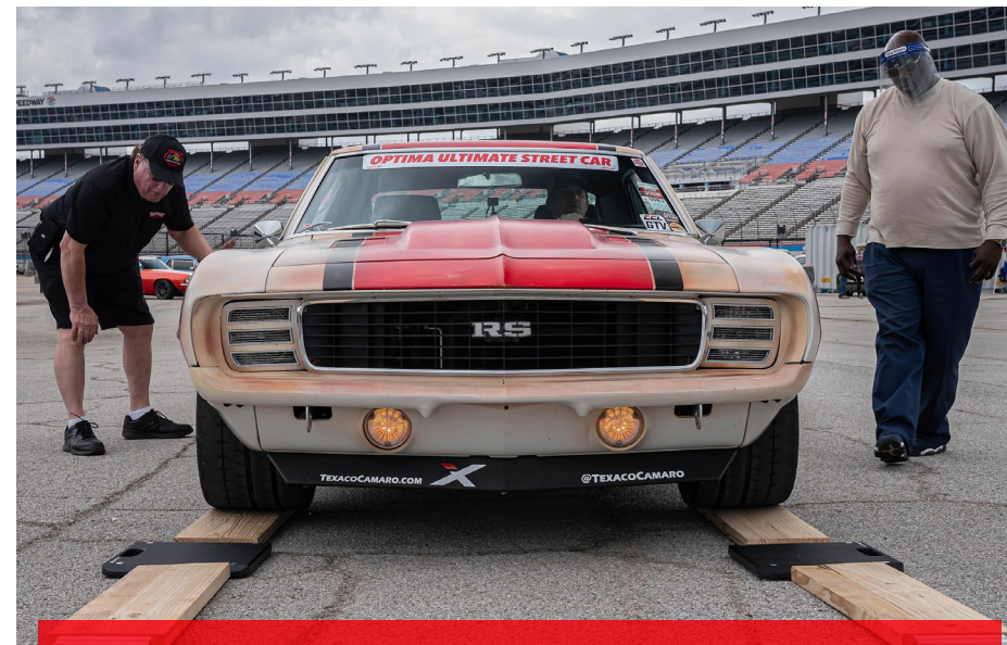
Vehicle scales play a key role in chassis setup across a range of racing disciplines. "For the teams in oval track, Formula Drift, and even drag racing, it's a cornerstone of race car setup," said Ryan Salata from PROFORM.
