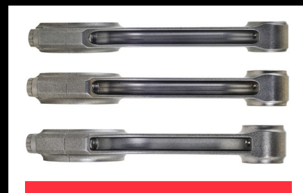
Pictured is a comparison of CP-Carrillo connecting rods with different offsets. From top, an LS rod that is on center, a small block Chevy rod with a .060-inch offset, and a small block Ford rod with a .110-inch offset.
