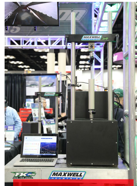
A shock dyno is almost mandatory in circle track racing's top tiers, reported Steve Watt from Maxwell Industries. Most teams put their shocks on the dyno between heat races and "check it again before the feature race."
