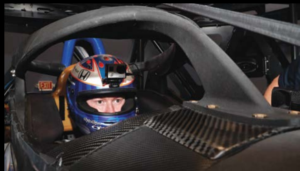
Development of IndyCar's monocoque safety cell included time in Dallara's driving simulator. Scott Dixon, seen here, tested the aeroscreen for proper sightlines.
