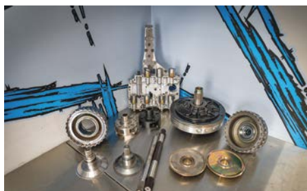
This photo from Rudy's Performance Parts shows some of a Ford transmission's stock hard parts next to Rudy's upgraded billet components, along with some of the prepped components ready for assembly, said Nathannial DeLong.
