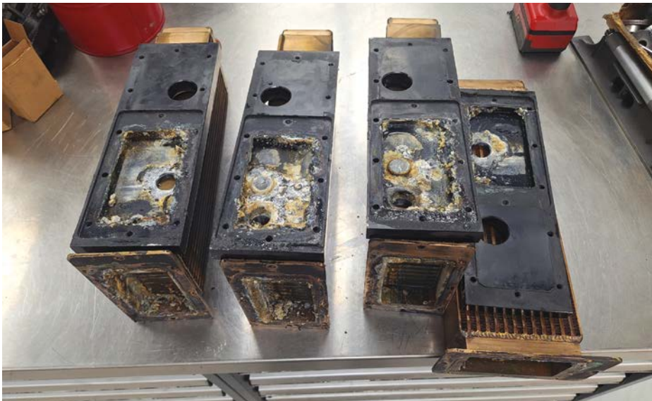
Marine racing is a "brutal environment," said Frank Beck of Beck Racing Engines, made worse by saltwater's corrosive effects. These intercoolers demonstrate just how much damage seawater can do to aluminum.
