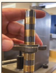
Custom Master gages for precise bore size and taper measurement.. accurate within 0.0001"
