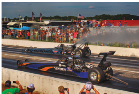
Dan Scheid (far lane) has been a pioneer in diesel drag racing, as his Top Dragster was one of the first in the 7s. He was a long-time proponent of making power with a lot of boost and no nitrous until just last year, when he added a modest (200–300 hp) nitrous system.
