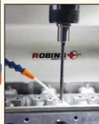
Guide honing upto 0.006" eliminates reaming .
