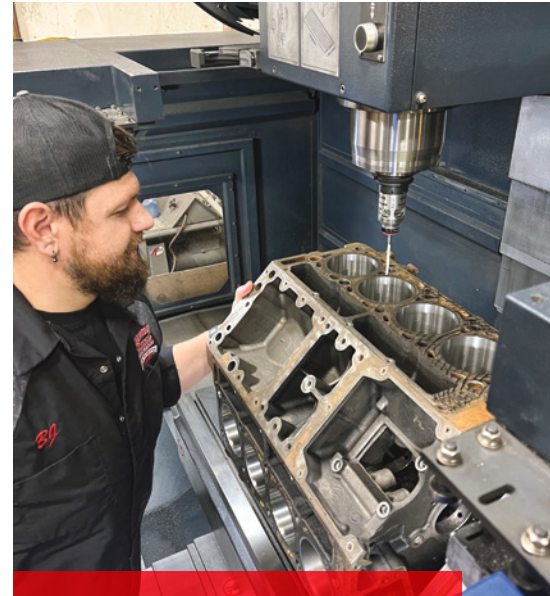
BJ Collins at Unlimited Diesel Performance watches the probe measuring the deck height on the RMC V50 machine center. Using its older equipment, “it would take us an entire day to bore and resurface a block,” said Nate Bailor. “When we bought the V50, I can bore eight cylinders in about eight minutes.”
