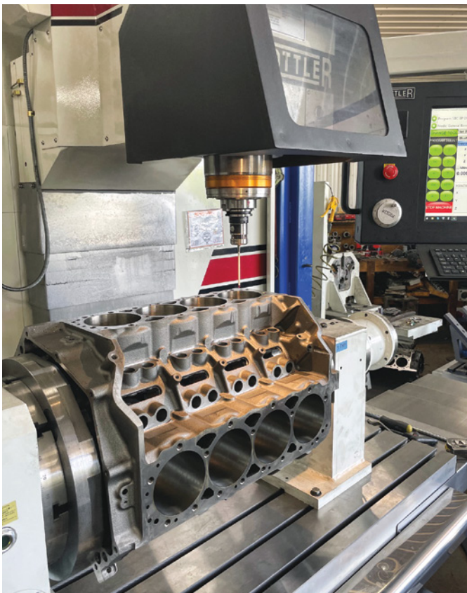
Pictured is an engine block set up on the Rottler F69A automatic machining center at Baldwin Racing Engines. Baldwin uses the F69A for line honing, cylinder boring, surfacing the decks, and lifter bores.
