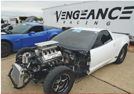
Ron Mowen describes the engine in the Vengeance Racing Corvette as "a miniature Pro Stock motor." The 451-cubic-inch LS engine produces about 1,140 hp and has propelled the car to a 199.7-mph top speed—so far.
