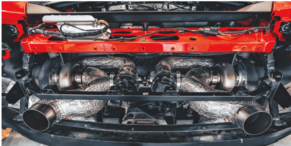
The V10 in Gintani’s Lamborghini Huracán EVO produced 630 hp in stock trim. Now twin turbocharged, the engine makes closer to 1,600 hp. It powered the Lamborghini to a blistering, 220-mph run in the standing half-mile last year.
