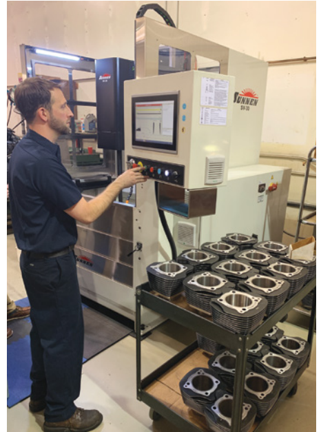
Engine builder and machinist Justin Bender works the Sunnen SV-30 honing machine at Zipper's Performance Products in Elkridge, Maryland. The shop fabricated a dedicated fixture that holds motorcycle cylinders for the honing procedure.
