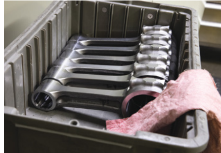
Connecting rods, like these from CP-Carrillo, are constructed with the bodies and caps married to each other. For the rods to function properly, it’s crucial that the caps and beams aren’t mixed during engine assembly.
