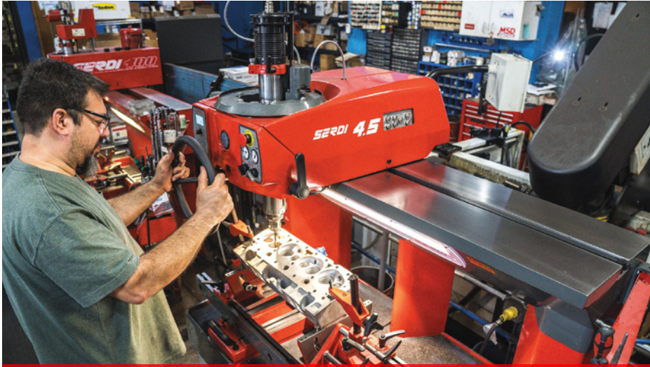
Don's Auto Parts and Machine Shop in Kenosha, Wisconsin, recently purchased a Serdi 4.5 seat-and-guide machine from RT Sales in Highland, Michigan. Adding this second Serdi machine to the shop will improve productivity, Tony Pontilla said, and enable him to hire more employees. Here, cylinder head tech specialist Hector Laracuente works on a head from a 410 winged sprint car engine.
