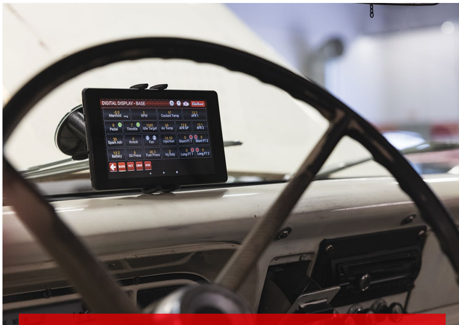
The enormous breadth of data-acquisition components available today allows these systems to be fitted to almost any vehicle imaginable—including older machines built long before the digital age.
